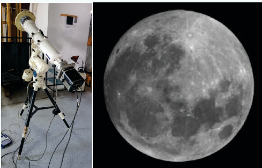
Figure 28. Left: 14-cm Vixen telescope with green line filter and CCD mounted for a test run at ARIES. Right: Sample image of the full moon captured around midnight during one of the exposure test runs.
