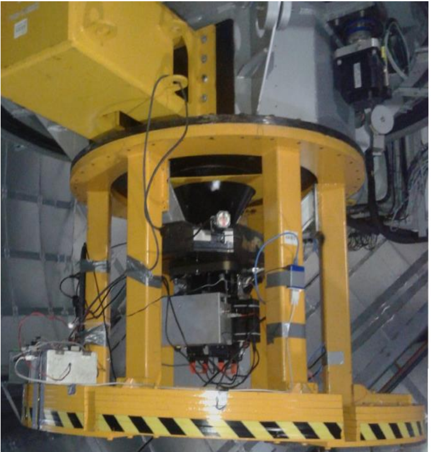
Figure 2: The 4Kx4K CCD camera along with the automated filter wheel as mounted at the axial port of the 3.6m DOT. Exposure time in a given filter and other CCD parameters could be set as per the science requirements. The Telescope could be operated both in open and closed loop modes using the auto-guiding unit through the Telescope Control Software. The details about making the telescope ready for observations and using the auto guiding units etc. will be provided through a separate set of documents/manuals. On site observing assistance will be provided. The user manuals of the CCD camera will also be provided separately to the observers. The instrument will be mounted/un-mounted by the observing assistants/staff members on duty in consultation with the instrument team.
