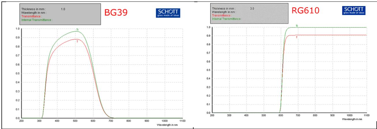
Transmission curves of the order-sorting filters, BG-39 and RG 610.
