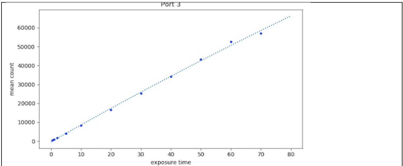
CCD signal linearity curve measured in the laboratory conditions. Presently, single port readout will be released. An IRAF script will be provided to users to make corrections for low-level non-linearity of the CCD response observed at low-light and bright-light conditions near saturation.
