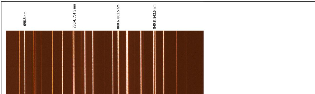
A portion of the Ar lamp spectrum recorded using the AD-FOSC.
