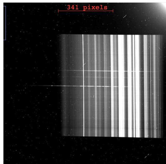
Fig 2b: Full spectrum (normal mode) through grism-300gr/mm without any filter. Slit is vertical and bright sky-lines can be easily seen.
