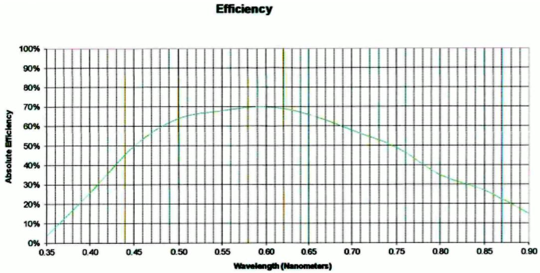
600 gr/mm (the wavelength axis unit is micrometer)
