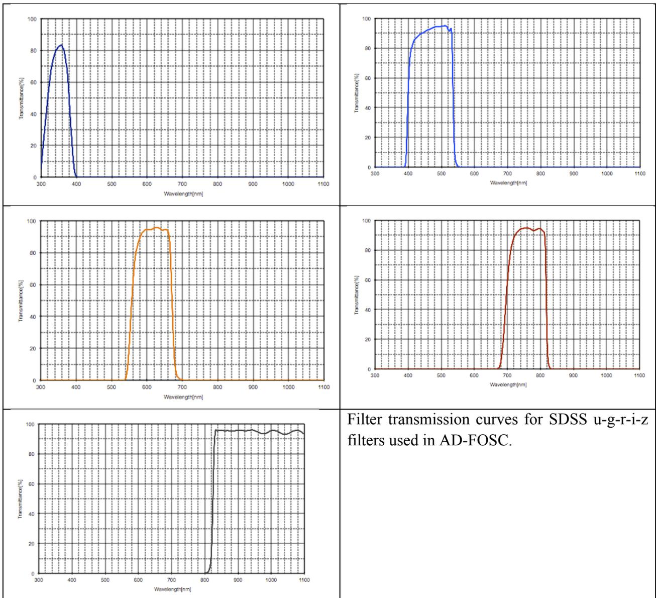
Filter transmission curves for SDSS u-g-r-i-z filters used in AD-FOSC.
