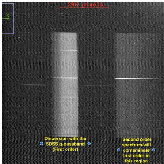
Fig. 2a: Spectrum through grism-300gr/mm limited by SDSS-g filter/ shows second order contamination region in first order space.
