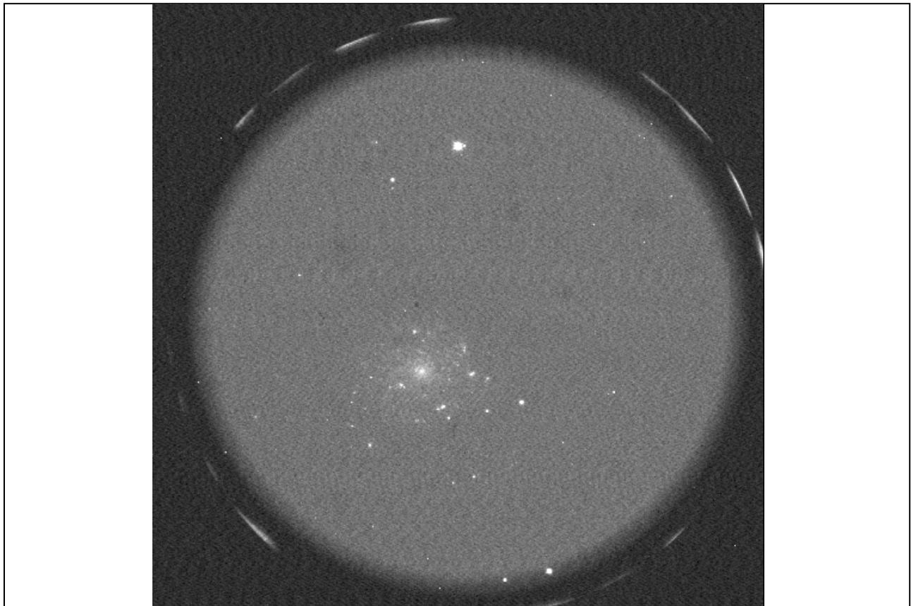
Fig. 3: Typical image taken in narrow-band filter. The available FoV is limited to 11' diameter.
