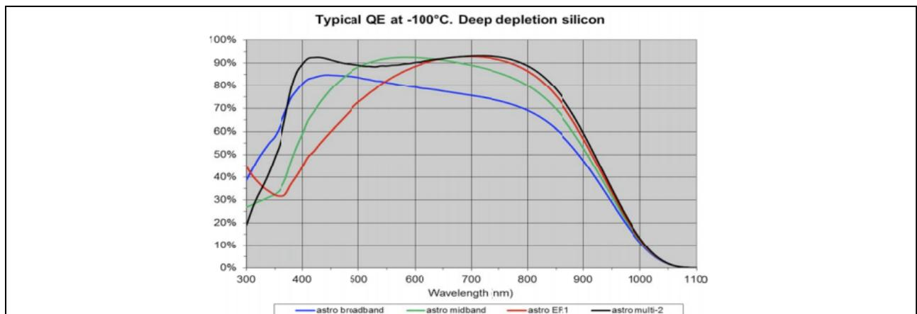
**Quantum efficiency:** ARIES 4Kx4K CCD camera uses E2V 231-84 version with astro multi-2 coating shown here by black curve.
