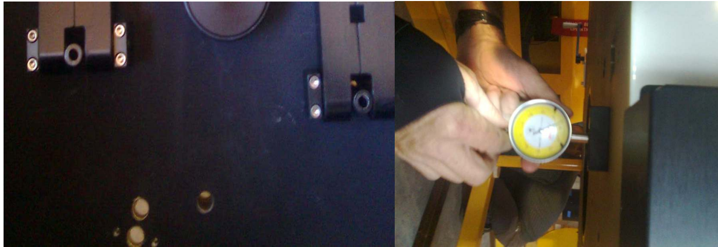
Figure 12: bottom central hole having two small holes both side is the position where we insert the dial gauges.
