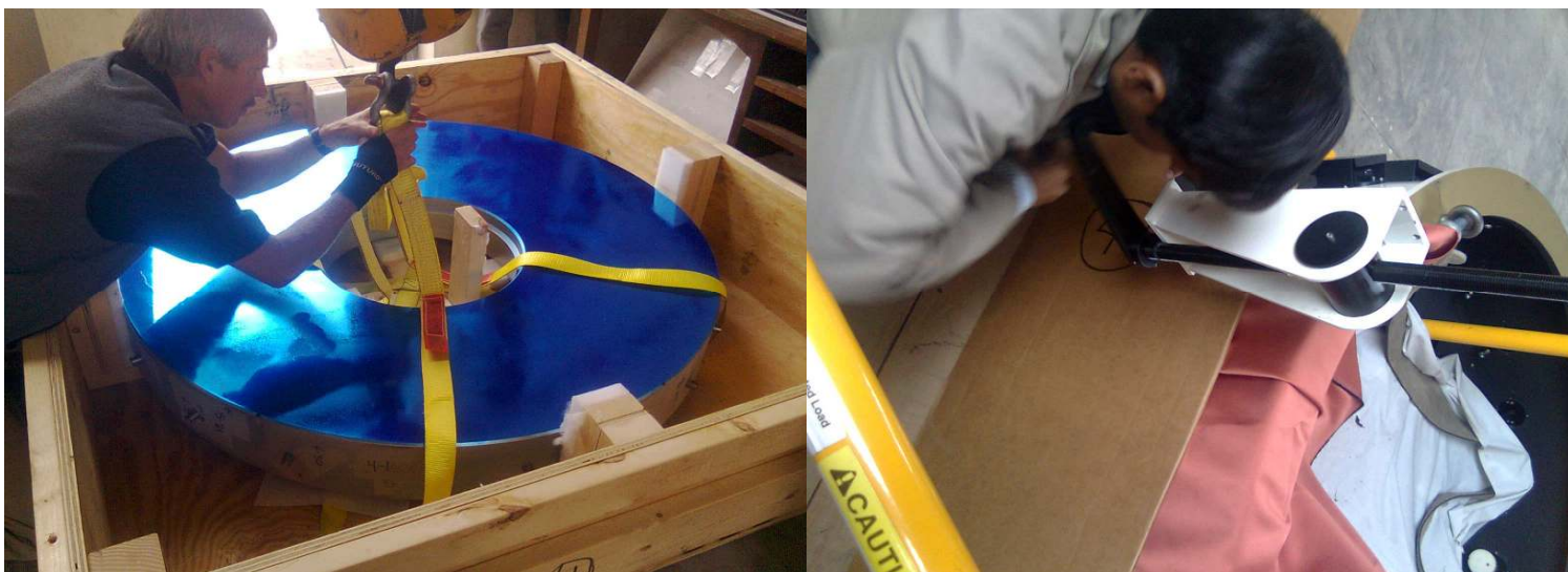
Figure 1: Fixing the sling on to the hook of the Crain (left) lifting the mirror cell using ratchet of MCLA(right)
