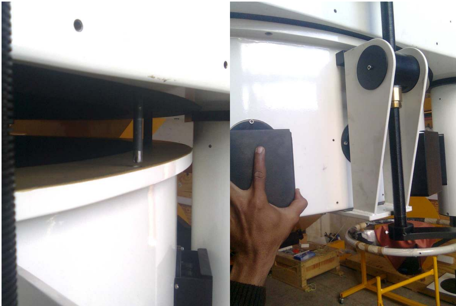
Figure 24: guide pin helping the cell to achieve best fit to the centre piece. Cell attached to the centre piece
