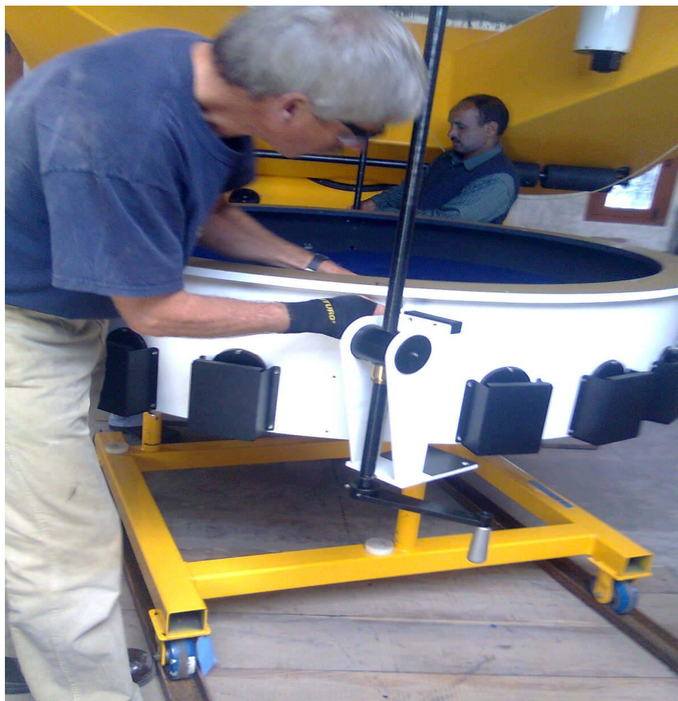
Figure 20: removing MCLA for placing earthquake guards.
