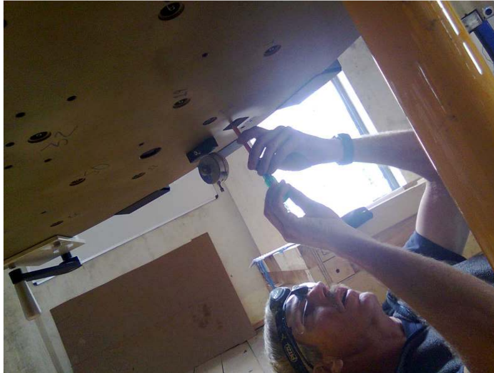
Figure22: tightening the screw (bottom brass nut, other two screw and a arm lock pin) of the axial definers
