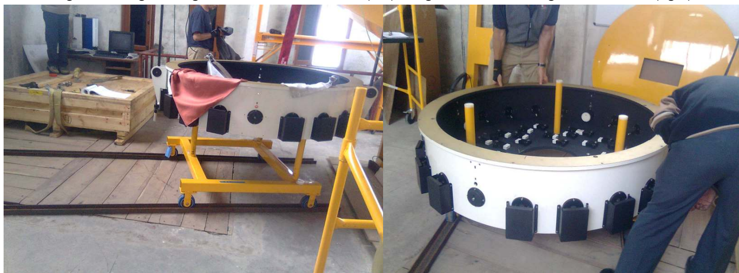
Figure2: mirror cell placed on top of mirror inserting tool and free to move on guiding rails; below centre section (left) at north west position (right)
