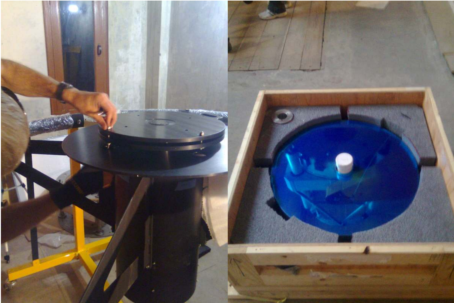
Figure 31: mounting the M2 plate in the spyder (left) M2 in its crate (right)
