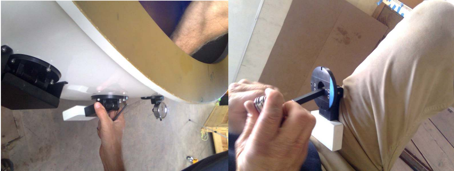
Figure 18: removing the counter weight assembly (left) putting a shim to fix the problem (right)
