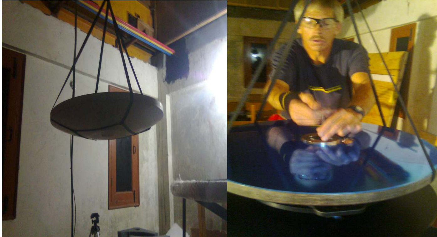
Figure 32: lifting the secondary mirror with Crain (left) fixing the secondary mirror hub to hold the M2 (right)
