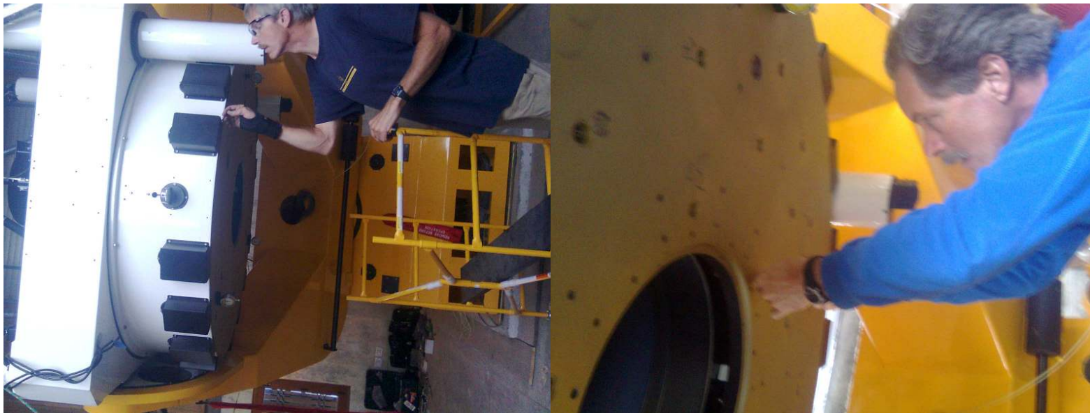
Figure28: checking the 16 radial counter weights (left) and 36 axial counter weights (right)
