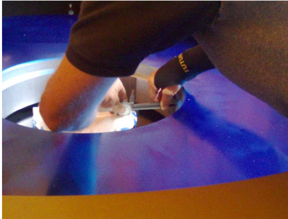
Figure 11: using a dial gauge from OD of corrector to ID of mirror.
