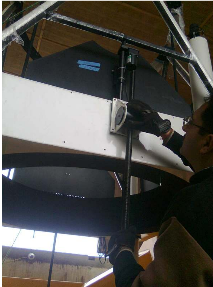
Figure 8: fixing the north MCLA (use two guide pins to fix this) *guide pins are pins used to fix in the holes provided for MCLA before putting MCLA and it allows you to have a comfort of easy hole matching.
