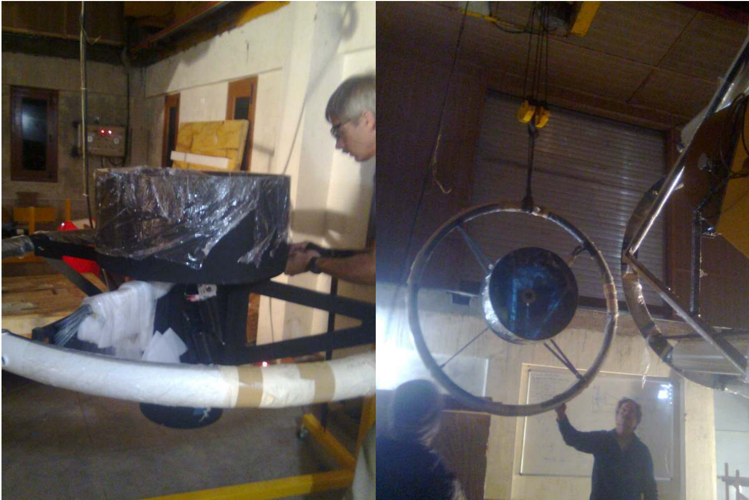
Figure 33: putting M2 baffle (light shield) (left) lifting the arrangement by Crain (right)
