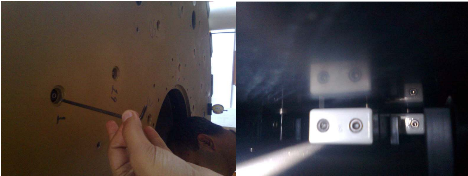
Figure26: placing the mirror on the 36 axial supports.
