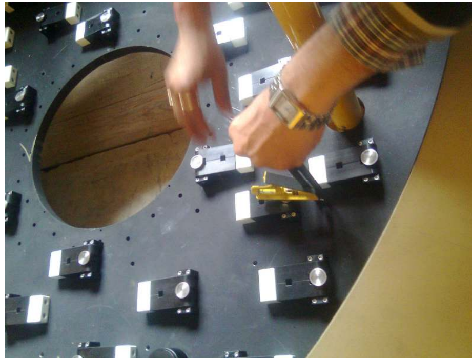
Figure 3: checking the height of all 36 axial supports and making sure that all tap pins are free
